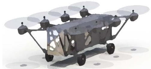
Figure 1 - The Multi-Mission Medical and CASEVAC UAV/UGV
