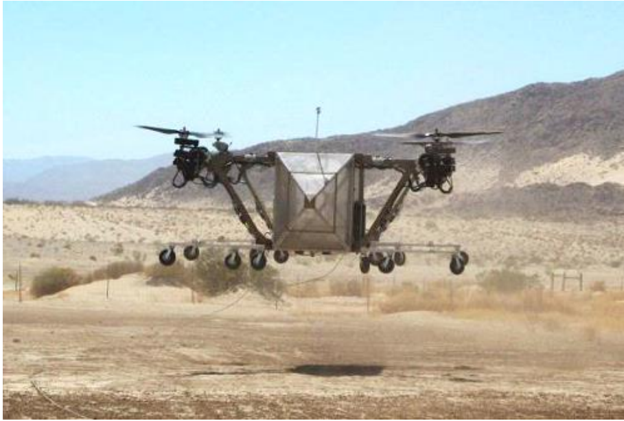
Figure 6 - Four-engine technology evaluation aircraft flown in 2012. It is gas powered and weighs over 2,000 lbs.
