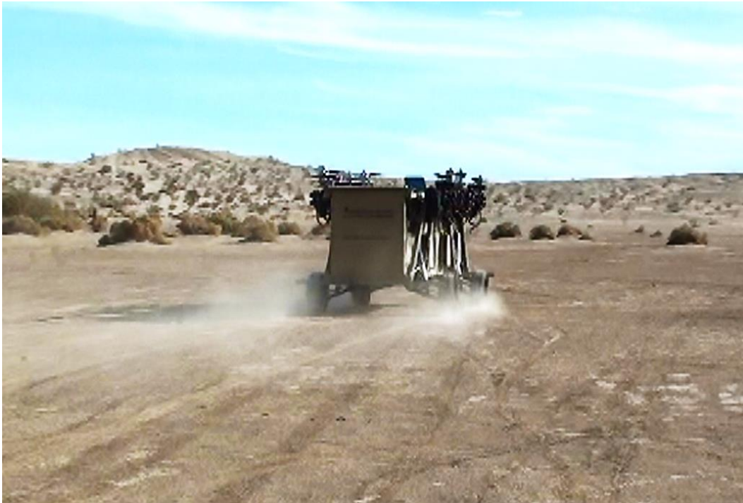
Figure 5 – AT Black Knight Transformer technology demonstrator during driving tests. The engines are stowed along the side of the vehicle to reach a street-legal width.
