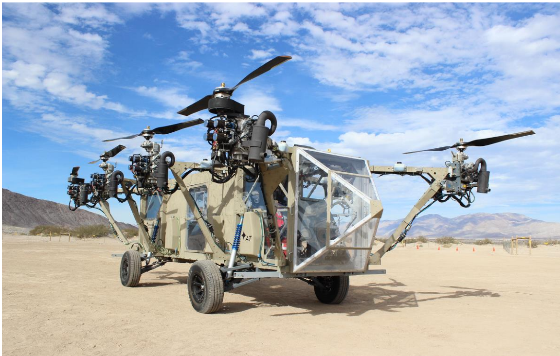
Figure 1 - The AT Black Knight Transformer, the world's first roadable VTOL aircraft. It is designed to be a low-cost rapid response ambulance to evacuate wounded soldiers from the battlefield or transport cargo.
