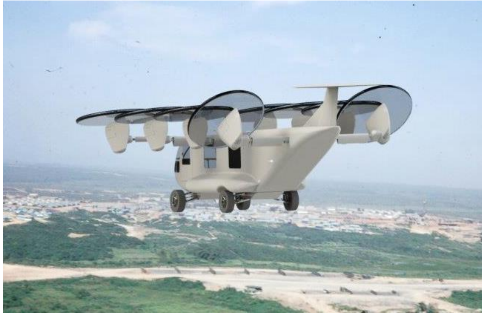
Figure 8 - Black Knight Transformer operational concept design with streamlined aerodynamics and more powerful and efficient turbo diesel engines.
