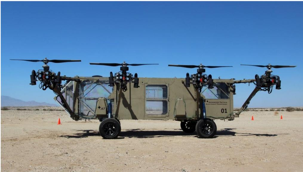
Figure 2 - The AT Black Knight Transformer has a large interior volume (similar to a BlackHawk helicopter) allowing it to transport cargo to the front lines and to carry wounded soldiers from the battlefield.
