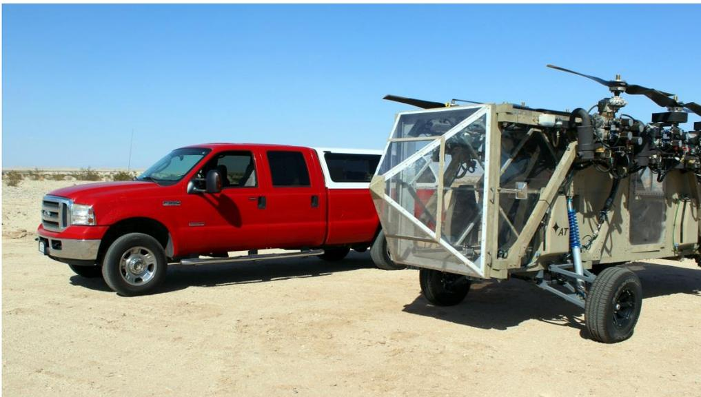
Figure 6 - The Black Knight Transformer is larger than a Ford F350 crew cab truck, shown for scale. The engines are stowed against the side of the vehicle in driving configuration.
