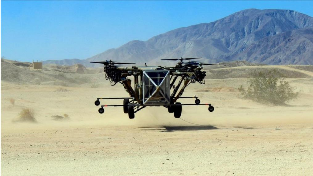
Figure 4 - The Black Knight Transformer during its first flight. Notice the attached electrical cable under the aircraft, which provided an emergency shutdown capability in case of a malfunction.
